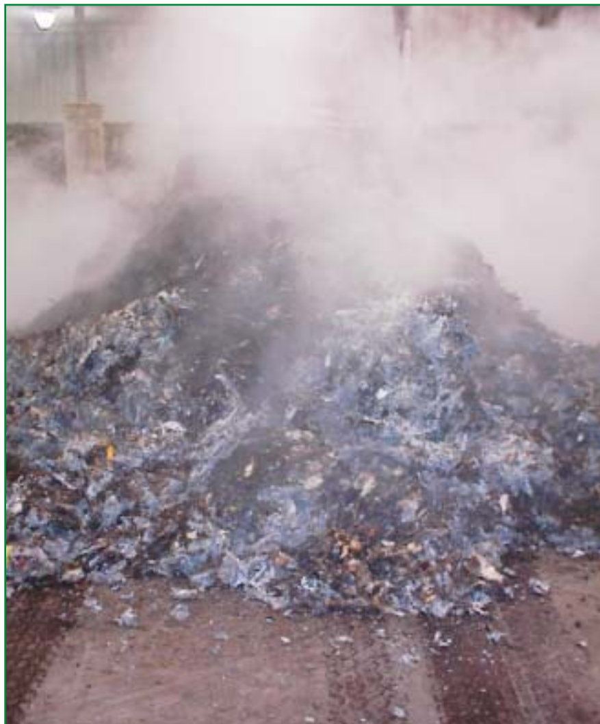
Bioaerosols are generated when a composting pile is agitated, particularly via mechanical mixing but also potentially via its mechanical aeration. The photo depicts bioaerosols at a Canadian composting facility.
