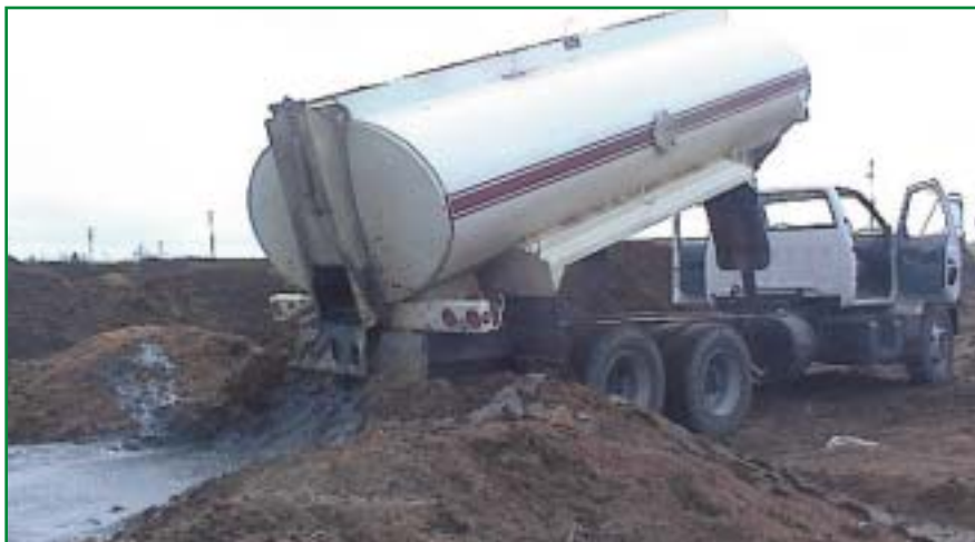
Devon sludge is emptied into a bunker of sawdust and woodchips. When the sludge is soaked up a compost pile is formed.
